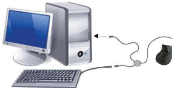
Figure 13. Connecting to the Host with Keyboard Wedge.
