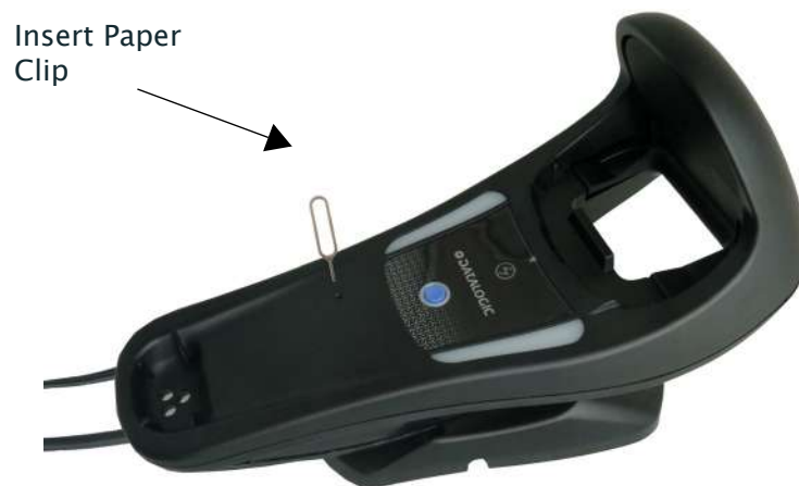
Figure 13 - Disconnecting the Cable
